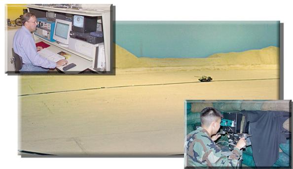
**Figure 6-6.** A Blaser tracking simulator with binocular viewing capability used at the Walter Reed Army Institute of Research in the 1990s.<sup>1</sup>
