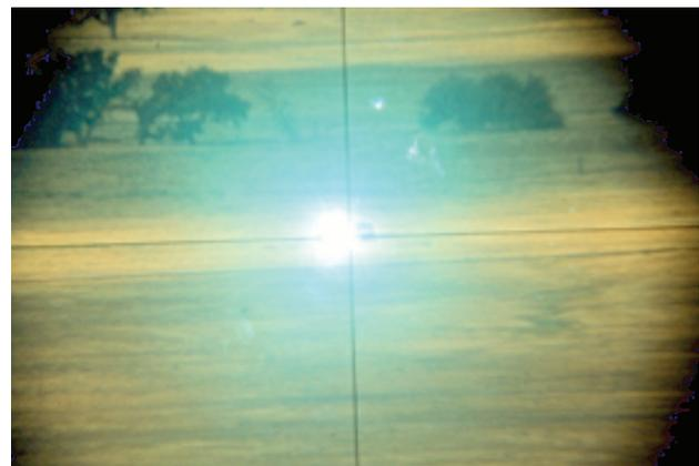
Figure 6-3. Laser glare veiling a target acquired through targeting optics. The veiling glare is from a laser source mounted on an armored vehicle directed at the viewing optics of a tube-launched, optically tracked, wire-guided missile system targeting the armored vehicle.
